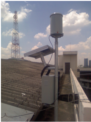
Figure 17: Wireless rain gauge system.
